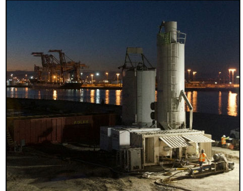
On-site Grout Batch Plant
