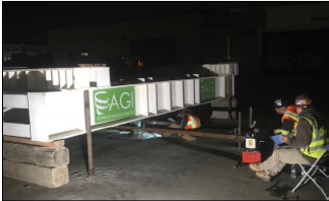
Compressive Load Test of Existing Wharf Piles
