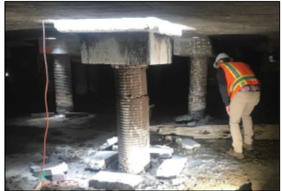
Plunging Failure Experienced During Compression Test
