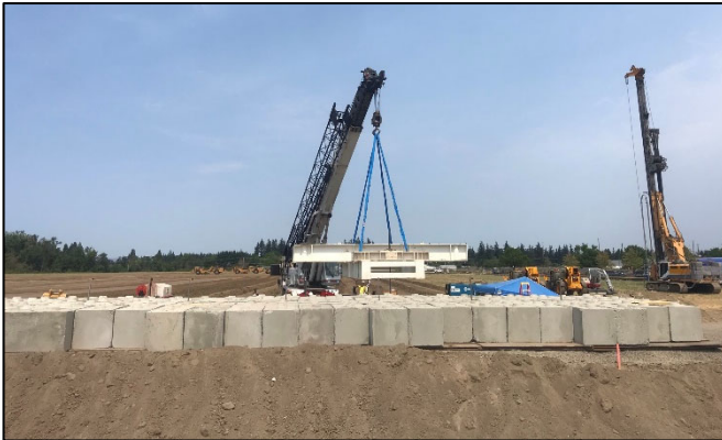
Slab-on-grade test area loading using ECO blocks and steel plates
