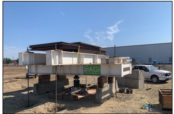
Compression load test of DSM column to 1,300 kips
